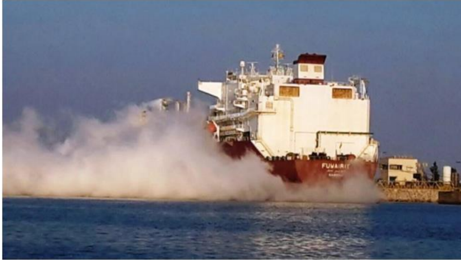
Figure 4. Formation of white cloud resulting from LNG spillage during vessel refueling (Kass et al., 2021).
